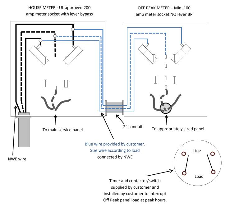
Northwestern Wisconsin Electric Company will supply wire to the top of the first meter socket. (BLACK WIRE SHOWN) All other materials on this diagram are supplied by the customer.
